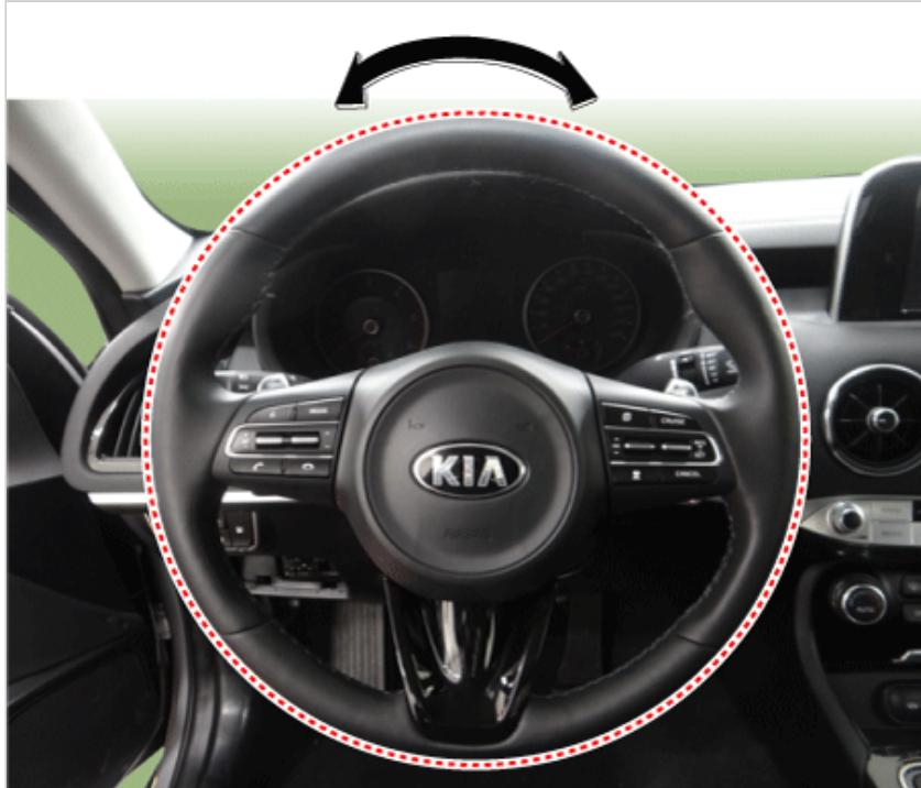
3. If the play exceeds standard value, inspect the steering column, shaft, and linkages.
